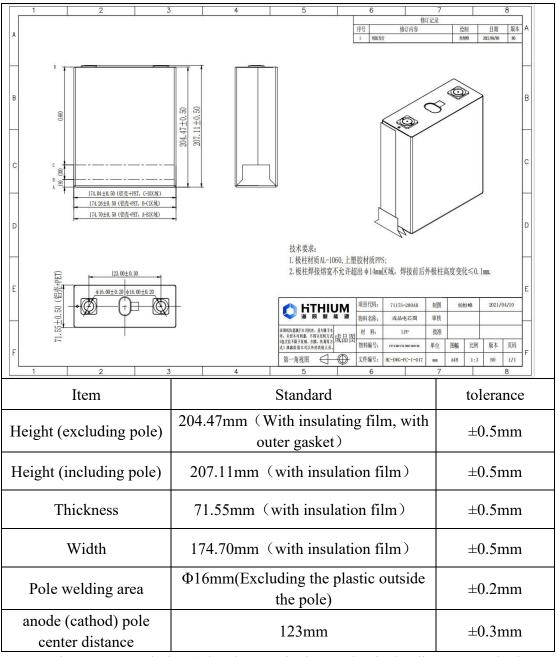
Note: Requirement Description (The size test is the mechanical splint test on the large surface of the battery, the initial preload is  $3000 \text{N} \pm 200 \text{N}$ .
